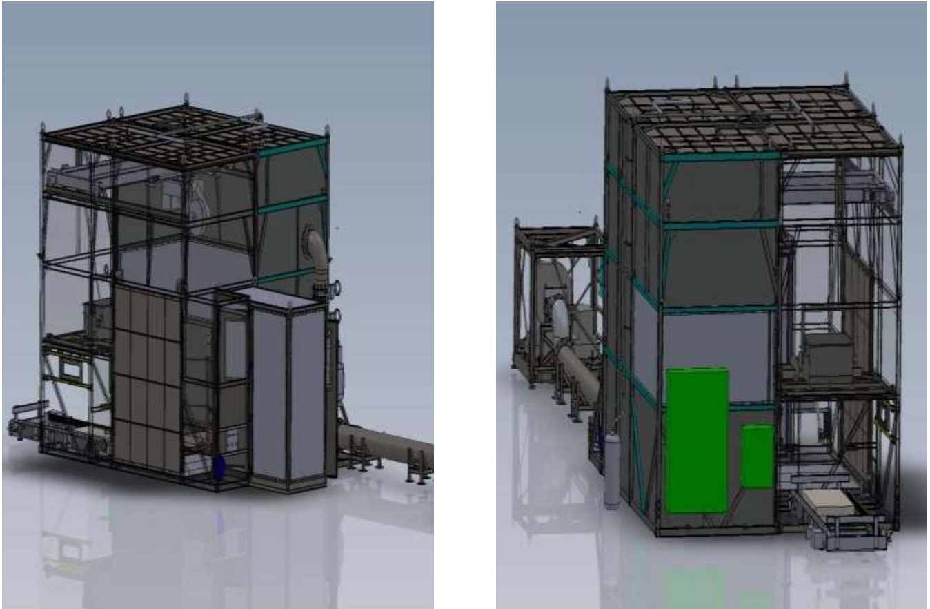
Fig.2. Solid radwaste extraction installation.
